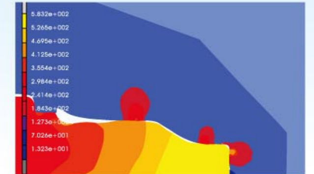
Stress distribution of shoulder and sealing surface after makeup (spherical surface is biggest and conic surface is smallest)
